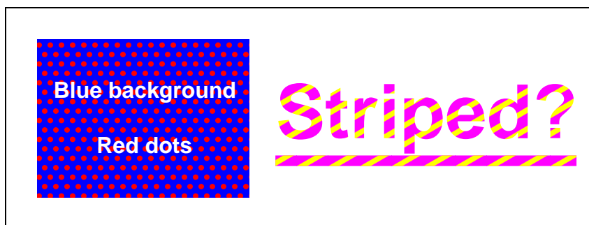
Figure 7: These are some examples for the above-mentioned pitfalls. On the left-hand side you should see a blue box with red dots and white text. On the right-hand side you see the underlined word "Striped?". Depending on your PostScript interpreter you either see a striped text, a striped underline, or both (filled with yellow lines on magenta background). The text may appear scrambled until you zoom in or print the document.
